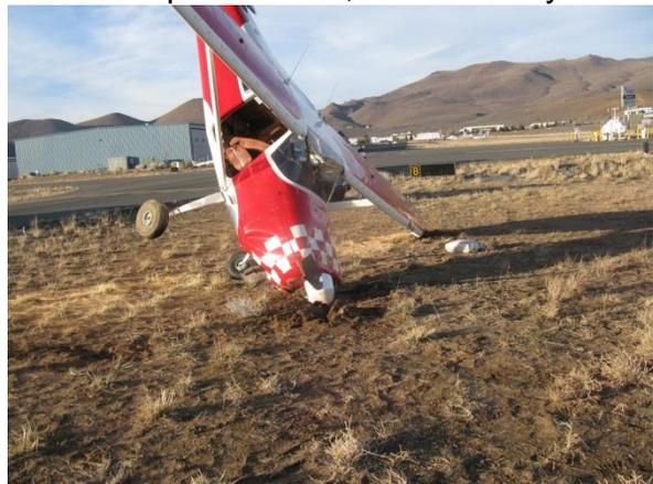
**Figure 1.** Airplane nosed over off of runway.
